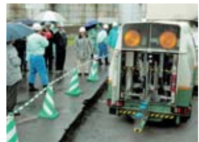
Test to use ash as roadbed (Kushiro Mill of Nippon Paper Industries)
