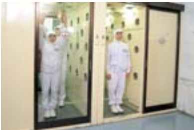
Air shower in an anteroom before entering the production area to remove foreign matter
